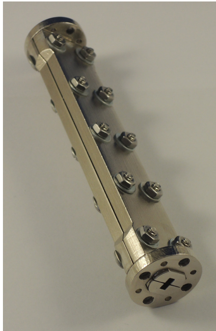
6. This is the assembled waveguide section prototype.
