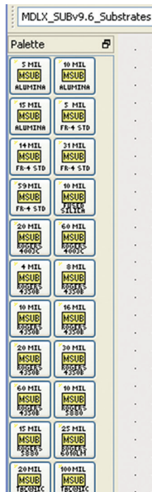
1. This substrate library is located in the palette's tab of an ADS schematic.
