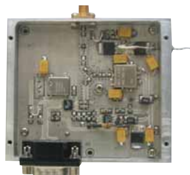
6. This photograph shows the fabricated 1.8-to-2.4-GHz frequency synthesizer.
