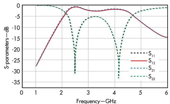
3. These are the simulated S-parameters of the CPW CRLH TL unit cell.
