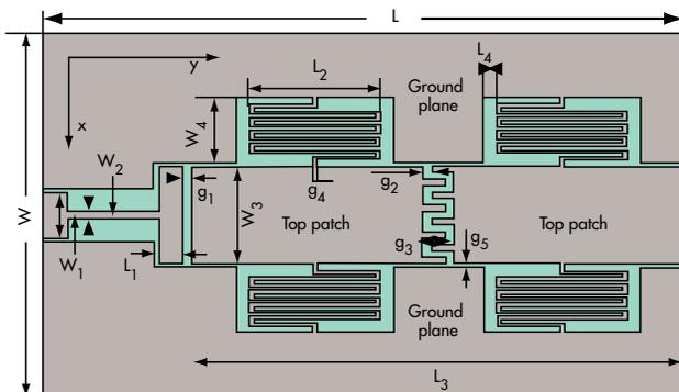
5. The top diagram shows the basic layout for a dual-frequency antenna based on a CPW CRLH TL unit resonator, while the photograph on the right is a fabricated CPW CRLH TL dual-frequency antenna.
