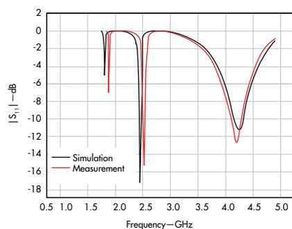
6. These plots show the simulated and measured return loss for the CPW CRLH TL dual-frequency antennas.
