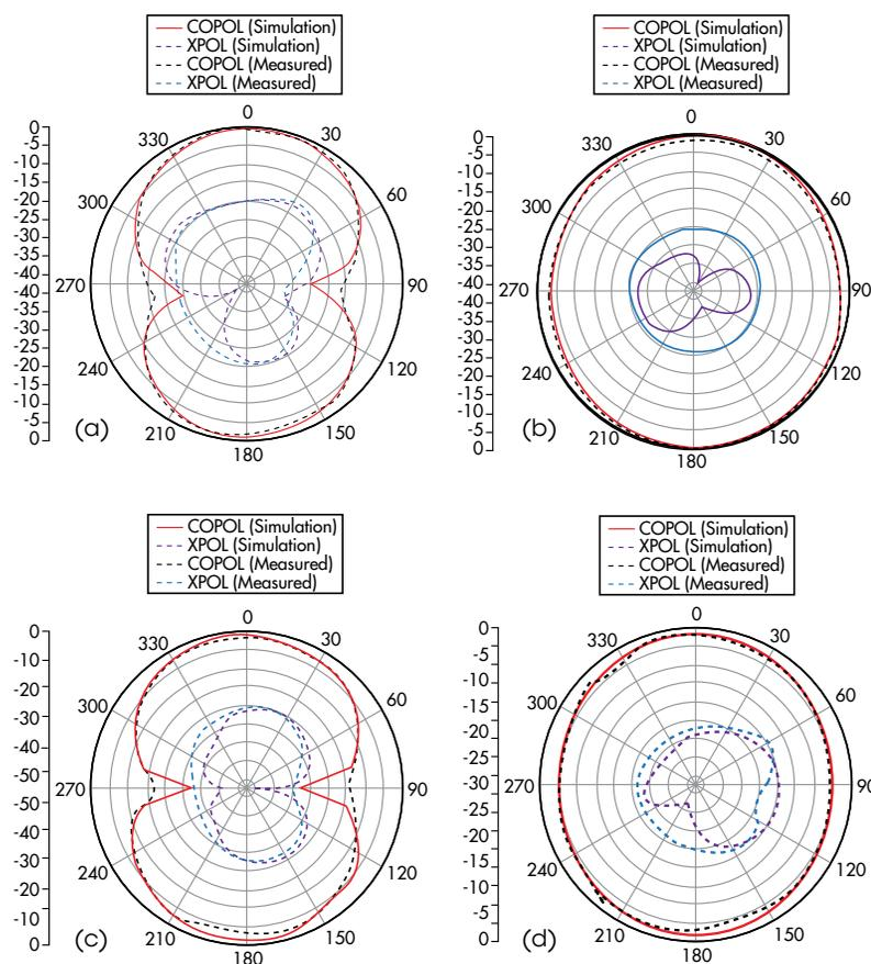
7. These simulated and measured responses show the antenna's zero- and first-order mode responses for its E- and H-plane patterns: (a) zero-order in E-plane, (b) zero order in H-plane, (c) first order in E-plane, and first-order in H-plane.
