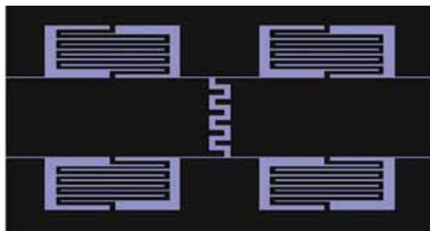
1. This diagram shows the basic structure of the CPW CRLH TL unit cell.
