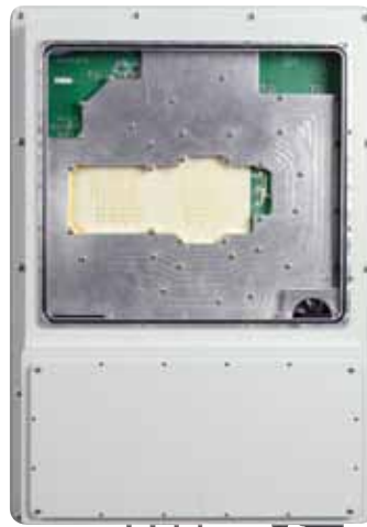
1. Prototype devices working at 28 GHz are designed to increase the data rates of next-generation wireless cellular systems. [Photo courtesy of Samsung ( www.samsung.com )]
