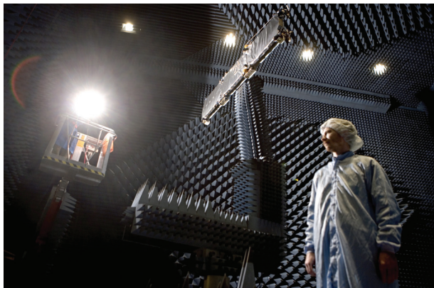
2. The Spherical Near-Field Antenna Test Facility (SNFTF) can test an antenna's behavior in the near-field and extrapolate far-field behavior using this data. (Courtesy of European Space Agency)
