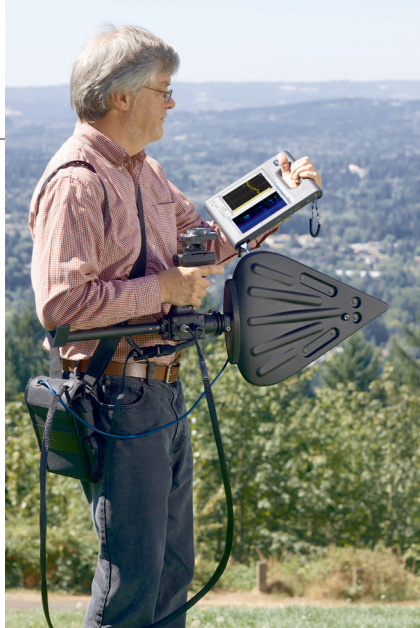
3. With its light weight and low power consumption, the RSA306 and the SignalVu-PC software can tackle a wide range of in-the-field measurements to 6.2 GHz.
