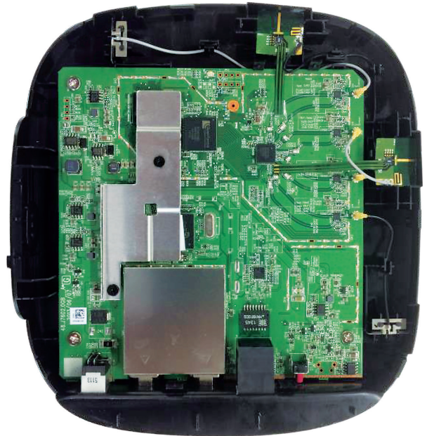
4. Active-steering antenna technology is beginning to be embraced for commercial technologies, such as enhancing Wi-Fi data rates, by eliminating dead zones and tracking high-demand devices. (Courtesy of Ethertronics)
