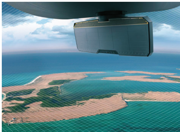
2. Using a modular approach to AESA construction can increase the scalability of a technology while easing integration into older platforms and technologies. (Courtesy of API Technologies)
