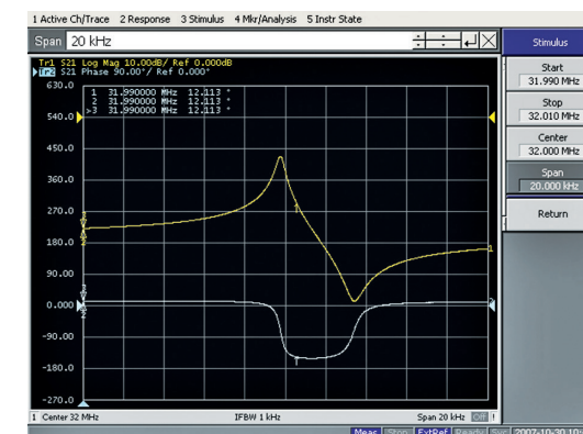
5. This is a network analyzer display for the negative group delay filter.
