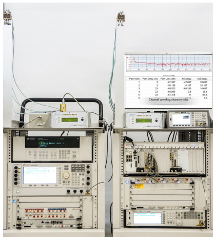
The 5G Channel Sounding Reference Solution test system incorporates PXI and AXIe measurement modules, along with flexible signal generation and analysis software, to tackle the challenges of characterizing 5G communications network channels.
