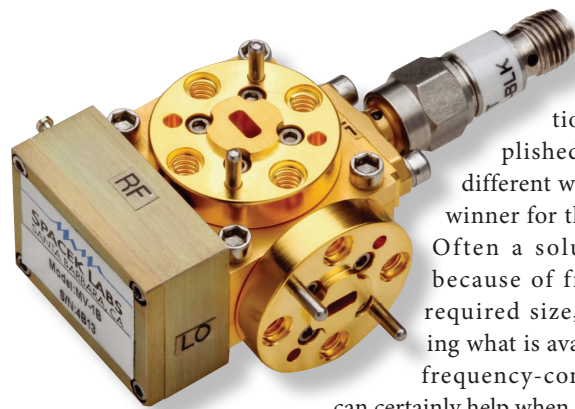
This mixer employs waveguide connectors for millimeter-wave frequency coverage and an SMA coaxial connector for an IF range of 10 MHz to 3 GHz. (Photo courtesy of Space Labs)
