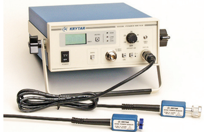
1. This traditional power meter and sensor combination provides power measurements from -39 to +20 dBm at frequencies from 100 kHz to 40 GHz. (Image courtesy of Krytar Inc.)
