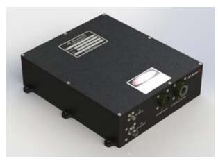
The dB-4150 MPM is a compact but robust wideband amplifier well-suited for wideband military applications in electronic-countermeasures (ECM) systems and electronic-warfare (EW) simulators. It is at home boosting either CW signals or signals with high pulse-repetition-frequency (PRF) pulse modulation. It can handle pulse widths as narrow as 1 µs through CW signals at maximum PRFs to 10 kHz.
