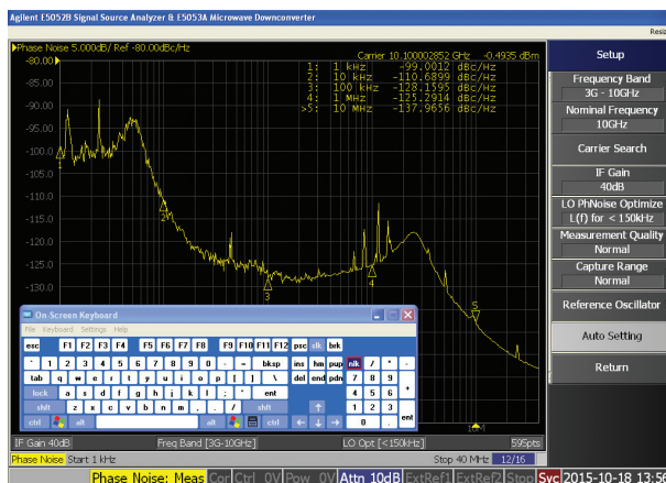
2. This plot shows phase-noise measurements on a 10.1-GHz carrier for a PHS-8400M frequency synthesizer. Testing is performed with a commercial frequency-downconverter and phase-noise test set from Keysight Technologies.
