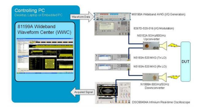
4. Among the test-equipment solutions targeting these specifications is the IEEE 802.11ad Physical Layer Signal Generation and Analysis System.
