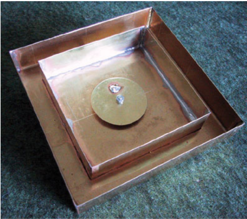
7. This simple radio-altimeter antenna is suitable for transparent fuselages.
