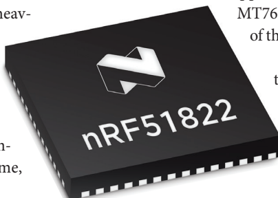
2. This single-chip 2.4-GHz device will find homes in Bluetooth Smart types of applications. (Courtesy of Nordic Semiconductor)
