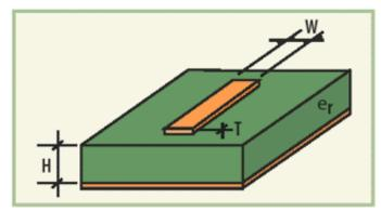
1. This simple cross-sectional diagram shows the basic dimensional parameters of a microstrip line on a printed-circuit board with relative dielectric constant  $\epsilon_r$ .
