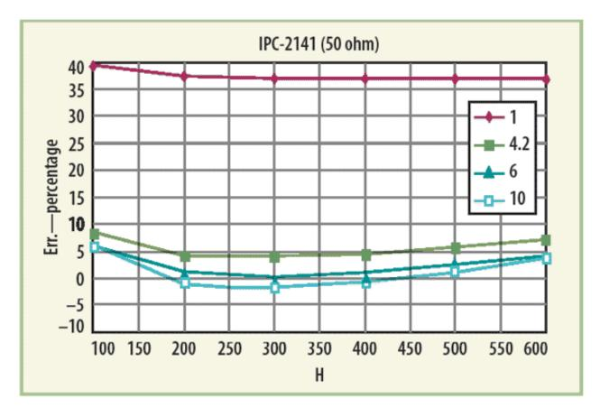
2. The expected errors for predicting W are shown as a function of H for the IPC-2141 50- $\Omega$  case.
