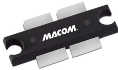
3. Plastic packaging is enabling a new generation of high-power modules.
