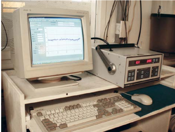
2. Manufacturing of high-performance SAW components requires computer-controlled automated measurements of SAW component performance. (Courtesy of Phonon Corp.)
