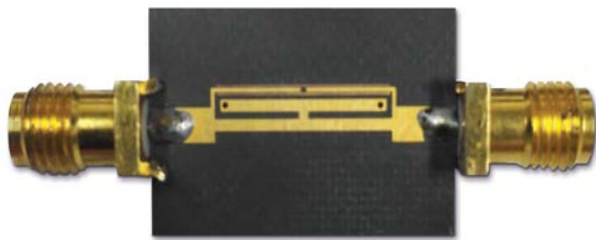
4. The UWB BPF was fabricated on 0.787-mm-thick RT/duroid 5880 circuit-board material (from Rogers Corp.) with relative permittivity of 2.2.
