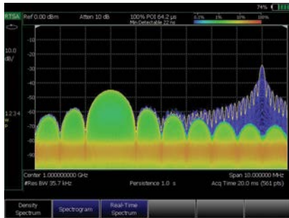
2. The portable FieldFox analyzers with optional RTSA capability can capture two simultaneous pulses and show traces on a bright, 6.5-in. diagonal TFT display screen.
