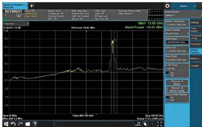
2. This screenshot shows the extremely wide span (10 MHz to 110 GHz in this case) that is possible with the N9014B UXA.
