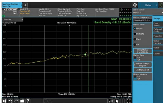
3. The wideband signal analyzer features impressive DANL, even for frequencies above 50 GHz.
