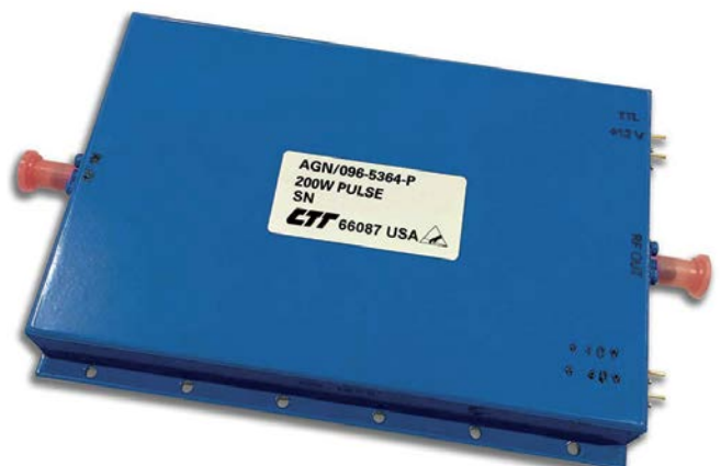
Thermal protection is built into this pulsed GaN PA, which provides 200 W output power from 8.5 to 9.6 GHz. The amplifier’s manufacturer emphasizes that the component must be used with a heat sink. (Courtesy of CTT Inc.)
