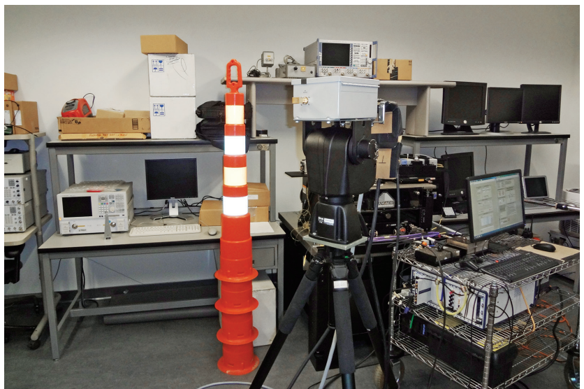
This photo shows the transmitter box used for channel-sounding measurements.
