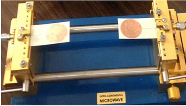
6. The photograph shows the measurement setup for the UWB antenna design, using a test fixture from Inter-Continental Microwave ( www.icmicrowave.com ).
