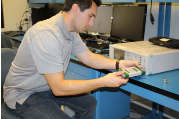
2. The Spectrum Master spectrum analyzers are small enough to connect directly to a DUT to eliminate the need for lossy, expensive interconnecting cables at millimeter-wave frequencies.
