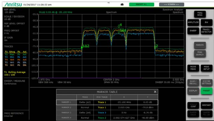
4. Markers can be placed where needed on signal traces to indicate measured values, with or without a trace marker shown on the screen to easily identify the markers.
