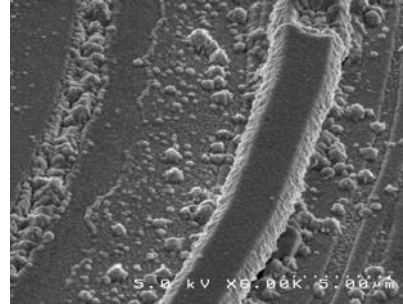
12. This SEM image shows that the width of the resonator ring was about 3 \mu\text{m} .
