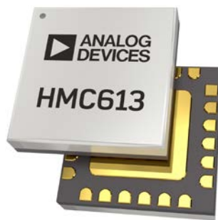
3. By leveraging semiconductor technology, this SDLVA (model HMC613LC4B) fits into a 24-lead, 4 × 4 mm SMT housing. It has a 59-dB logging range from 100 MHz to 20 GHz. (Courtesy of Analog Devices.)
