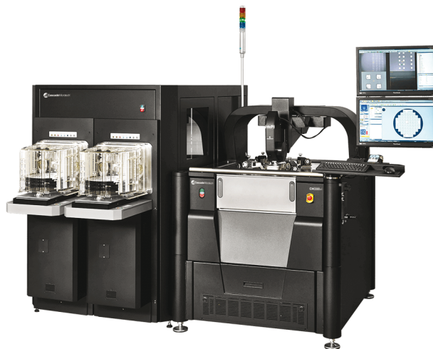
1. The CM300xi probe station features micro positioners under computer control to achieve submicron positioning resolution and accuracy when placing a test probe on a circuit. (Courtesy of Cascade Microtech)
