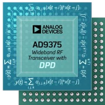
1. The AD9375 RadioVerse transceiver contains a fully integrated DPD solution, two differential transmitters, two differential receivers, an observation receiver, and a sniffer receiver with total frequency range of 300 MHz to 6 GHz in a compact BGA package.
