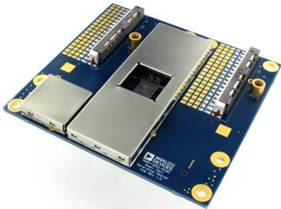
2. The AD9375 small cell radio reference design helps system designers working on 3G, 4G, and 5G small cells to come to market quickly with a low-power radio design characterized for LTE use.
