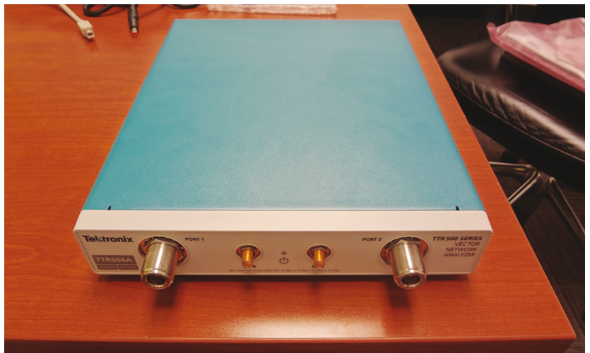
1. Shown is a photo of the actual VNA used to perform the measurements described throughout this article.
