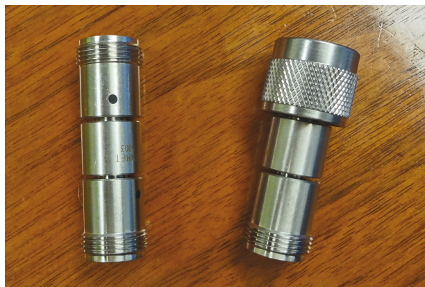
7. Shown are the adaptors used to perform calibration and measurements, respectively.
