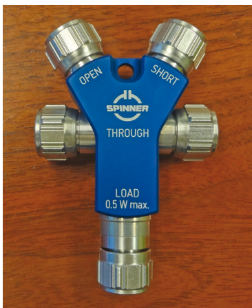
4. This figure shows the calibration kit used to calibrate the VNA.
