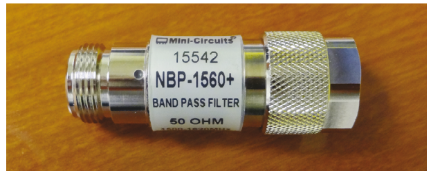
3. Shown is the actual bandpass filter that was used as the DUT.
