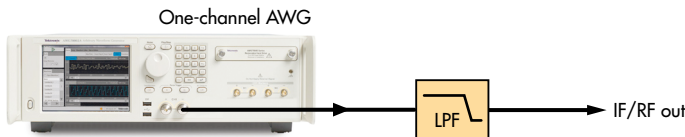
(c) Direct RF generation in the second Nyquist band
