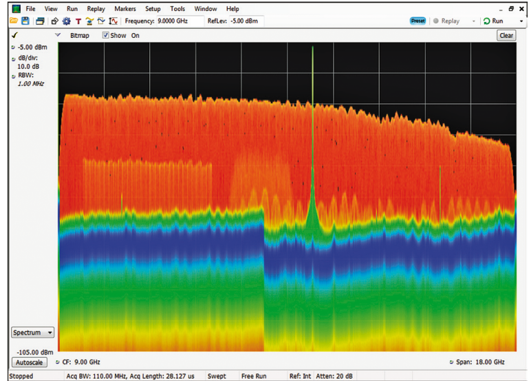
2. With its high-speed digital-to-analog signal conversion architecture, a modern AWG is capable of producing a wideband signal environment suitable for radar system testing.
