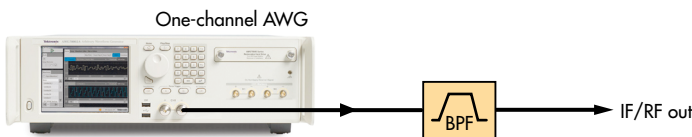
(c) Direct RF generation in the second Nyquist band
