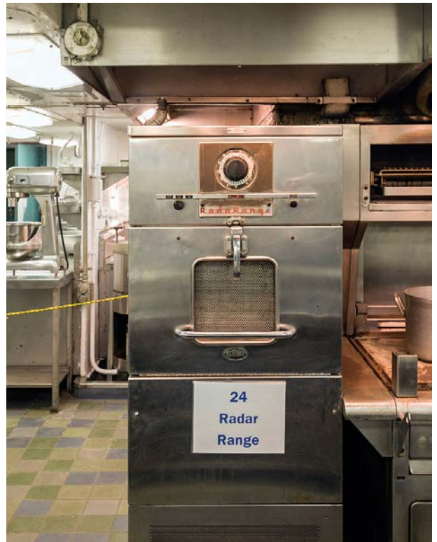
1. A Raytheon Radarange was installed on the NS Savannah nuclear-powered cargo ship (now a museum ship) in 1961 (Source: Wikipedia)
