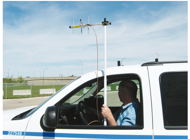
1. SaskTel interference hunters use “broomstick” antennas and USB-based real-time spectrum analyzers to track down sources of interference.
