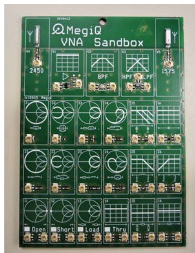
2. This is a photo of the VNA Sandbox, which contains a variety of RF circuits.
