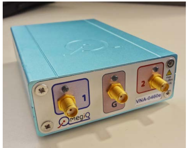
1. This is the VNA included in the demo kit. It covers a frequency range of 400 MHz to 6 GHz.
