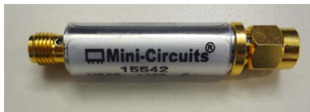
7. Shown is the SMA-connected bandpass filter used as the DUT.
