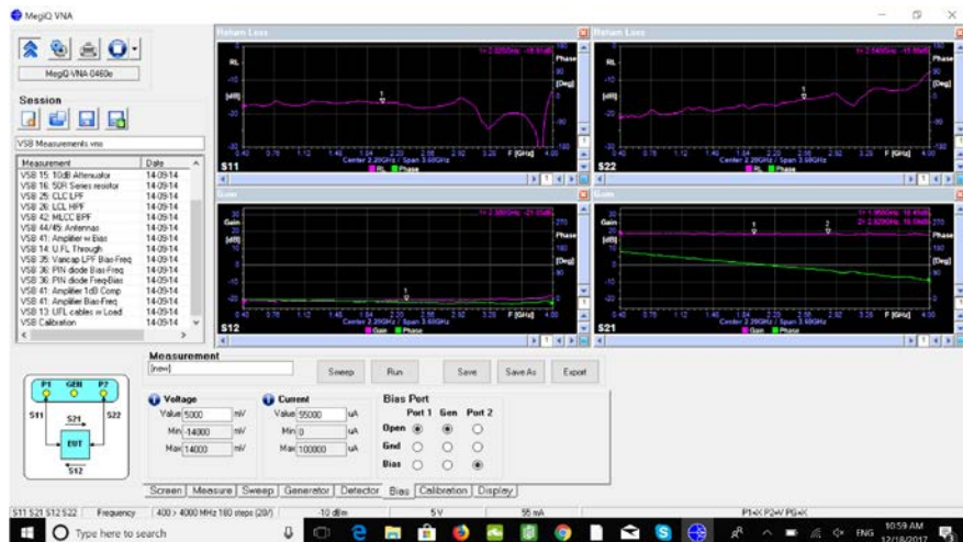
5. The amplifier was measured by utilizing the VNA's internal bias generator. Shown is the measured data.
