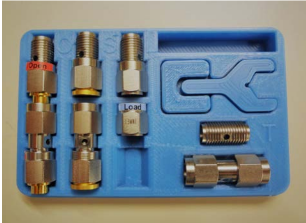
8. This photo shows the SMA calibration kit that was included with the demo kit.
