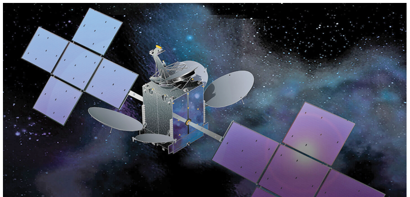
1. Artificial satellites were once entirely geosynchronous-earth-orbit (GEO) types at high altitudes and with larger cover areas, but the current trend is for using larger numbers of smaller low-earth-orbit (LEO) satellites at lower altitudes and smaller coverage areas. (Courtesy of Telesat)
