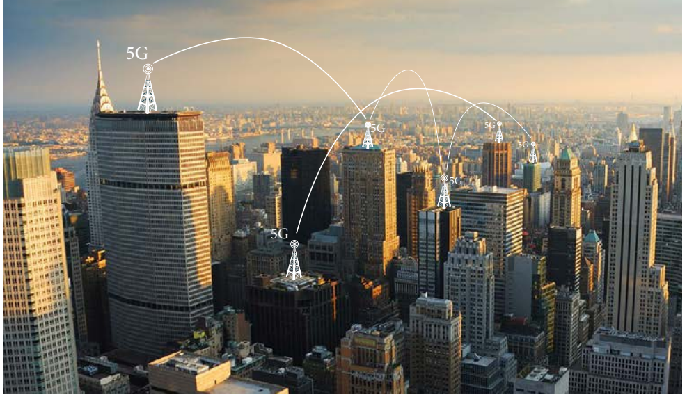
2. The infrastructure for 5G wireless networks will employ many more closely spaced base stations than earlier wireless networks, to support the shorter propagation distances of mmWave signals. (Courtesy of Verizon)
