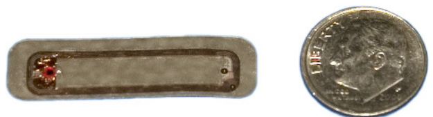
8. Conventional RFID tags can be supplied in extremely small sizes for unobtrusive attachment to the metal surfaces of firearms.
