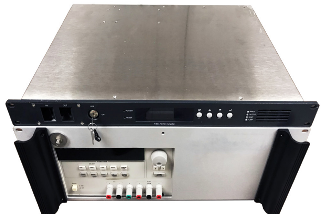
1. Shown in two views, this line of rack-mountable frequency synthesizers employs different techniques and technologies to trim phase noise at X- and K-band frequencies.
