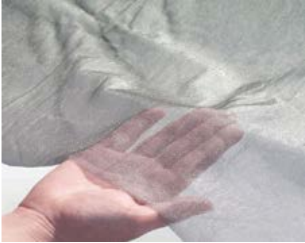
1. Lightweight silver/polyamide mesh shielding materials are capable of 50 dB or more shielding. (Courtesy of AaroniaUSA)
