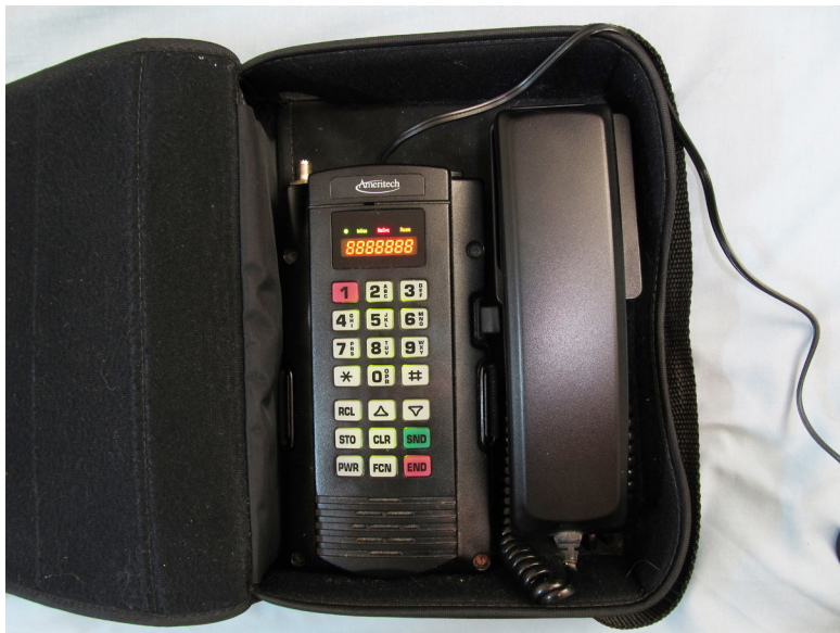
Early mobile cellular telephones used analog transmission techniques in 1G systems, switching to digital switching in the following generation. (Courtesy of Wikipedia)
