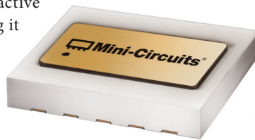
2. The MAC series of surface-mount mixers makes use of LTCC technology and monolithic active devices to achieve high-performance mixers in tiny hermetic packages. [Photo courtesy of Mini-Circuits ( www.minicircuits.com )]
