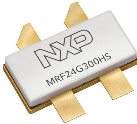
1. Model MRF24G300HS is a high-power GaN-on-SiC transistor developed for CW and long-pulse application from 2400 to 2500 MHz, and as a solid-state replacement for magnetrons at 2.45 GHz in heating and welding systems. (Courtesy of NXP Semiconductors)
