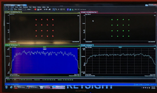
4. This is a wideband research-and-development mmWave test bed with a four-channel 110-GHz UXR.
