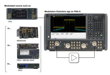
1. MOD is a software application that runs on the PNA-X. It provides an innovative approach for performing device characterization under wideband modulated signals.
