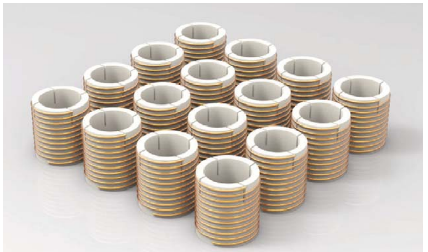
1. Schematic of the magnetic metamaterial: The metamaterial array composes unit cells featuring metallic helices, which are made of copper wiring with central polymeric scaffolding (scale bar is 3 cm). (Source: Boston University)
