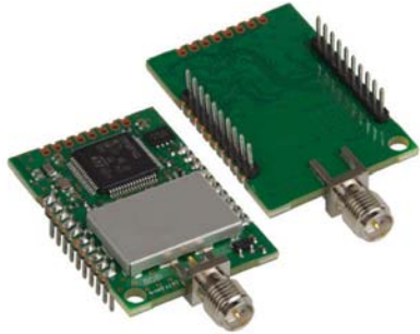
MultiTech's mDot module uses an Arm Mbed processor to provide LoRaWAN connectivity for M2M applications.
