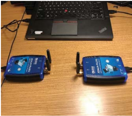
8. The SDR configuration uses ADALM-PLUTO radios (left). Also shown is a corresponding confusion matrix (right). (© 1984–2019 The MathWorks, Inc.)
