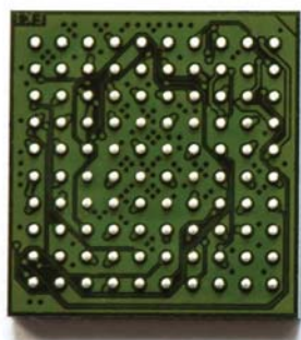
1. zGlue's Smart Fabric silicon interposer technology allows chiplets to be mounted within a chip to deliver compact, custom chips.
