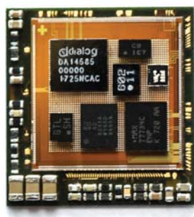
1. zGlue's Smart Fabric silicon interposer technology allows chiplets to be mounted within a chip to deliver compact, custom chips.
