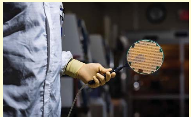
GaN and GaAs 6-in. diameter semiconductor wafers are part of a foundry that serves both military and commercial customers.
