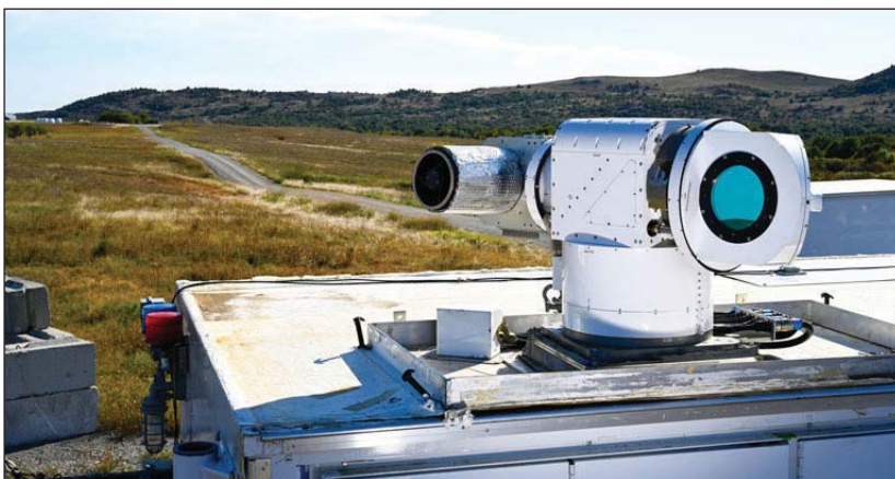
4. The ATHENA system is a HEL-based DEW designed as a defense against drones. (Courtesy of Lockheed Martin)
