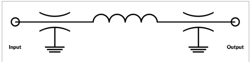
8. A π (Pi) circuit is two "C" circuits separated by a series of inductive elements.
