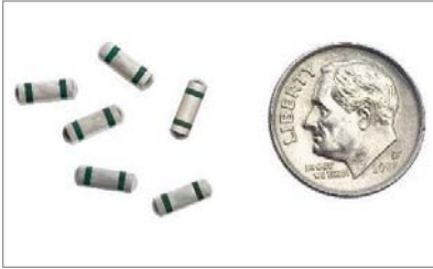
10. SMT filters have a maximum capacitance of 8,200.
